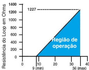
$$Vdc \text{ MIN} = 9V + [0,22A \times R_L]$$
